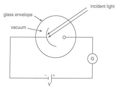
The diagram above shows a simplified arrangement to demonstrate the photoelectric effect. The equation usually associated with this phenomenon is  $E_K = hf - \Phi$ , where  $E_K$  is the kinetic energy of any released electrons and  $\Phi$  is the work function of the metal being used.
