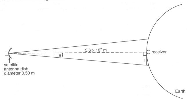
(f) The distance above the Earth's surface of the satellite is  $3.6 \times 10^7$  m, the wavelength of the transmitted wave is  $1.0 \times 10^{-3}$  m and the diameter of the antenna dish is 0.50 m.
