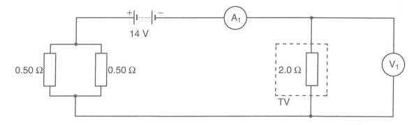
(b) (i) Determine the effective total resistance of the circuit.
